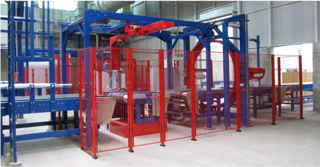
To meet the increasing demand for middle speed waste bale wrappers, REO-PACK has launched the new W1000 wrapper. The W1000 can wrap both horizontally and vertically at the same time, without turning the bale, this give a unique flexibility and high efficiency.
