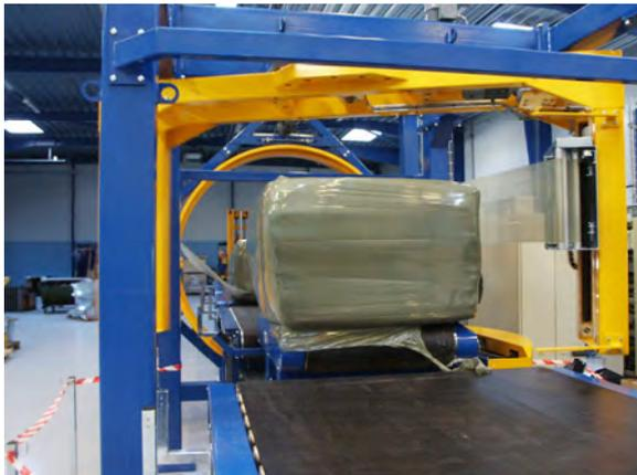
**STEP 1:** Horizontal wrapping in the W1000 swing arm wrapper.
