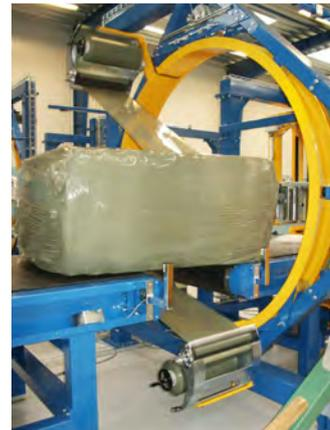
**STEP 2:** Vertical wrapping in the vertical ring wrapper.
